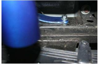
6. Fit 1 x bolt on wire on either side in through chassis and out through retainer hole in Kaymar bar using M12 flat, spring and nut. DO NOT TIGHTEN.
