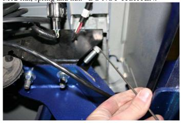
7. Fit bolt plate into chassis down through support gusset in Kaymar bar using M12 flat, spring and nut. DO THESE BOLTS UP FIRST.
